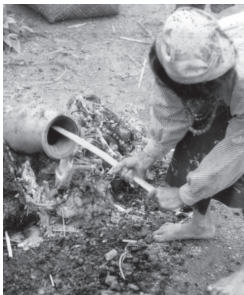
The pot is sun-dried and then fired with corn cobs and kindling.
