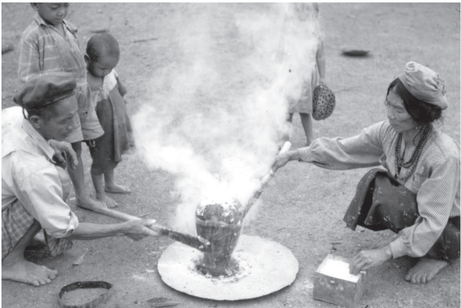
The hot pot is glazed with cimh powder, from the sap of a tree called cingh sing .
